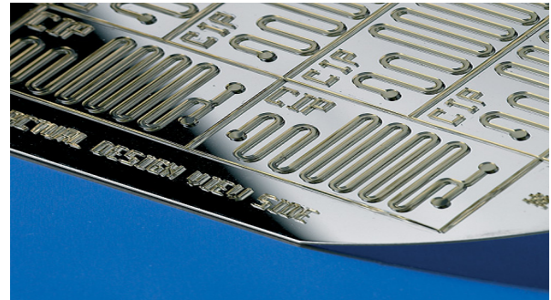
Figure 4: SU-8 positive mould
